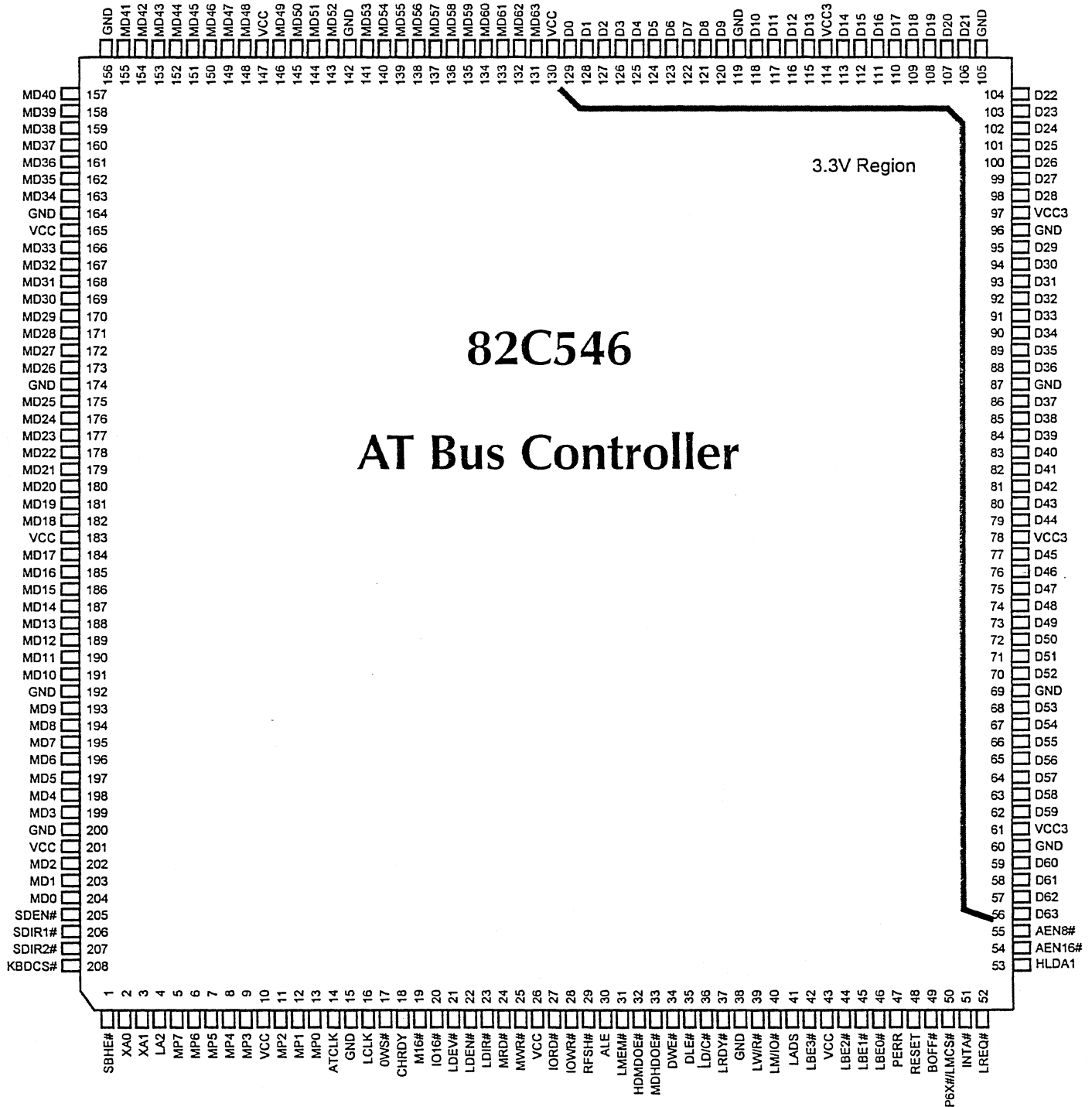
Figure 3-1 82C546 ATC Pin Diagram
