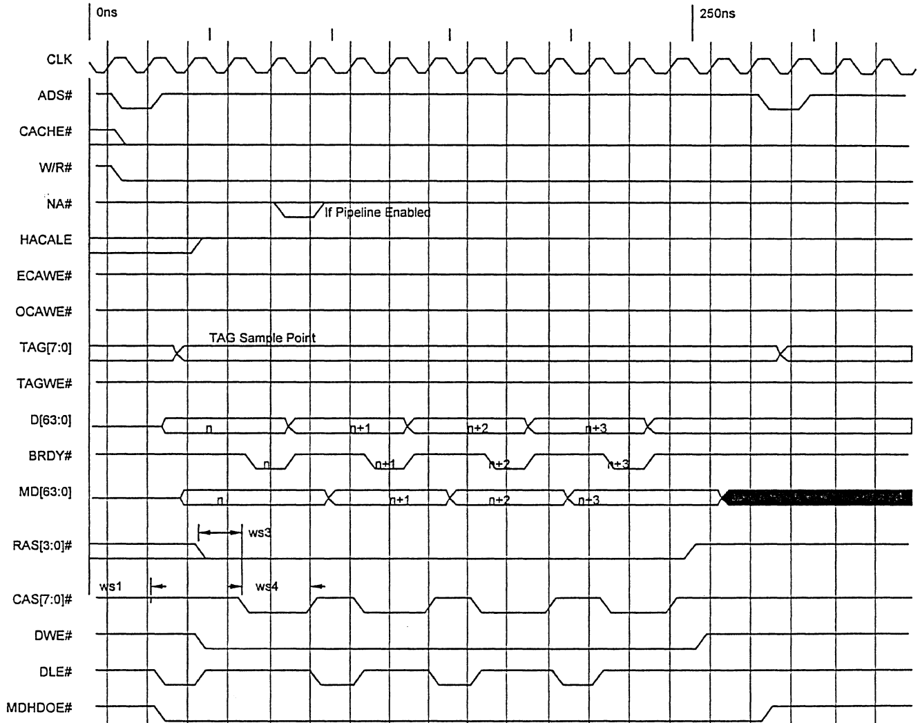
Figure 4-10 L2 Cache Write-Miss Burst (4-3-3-3)
