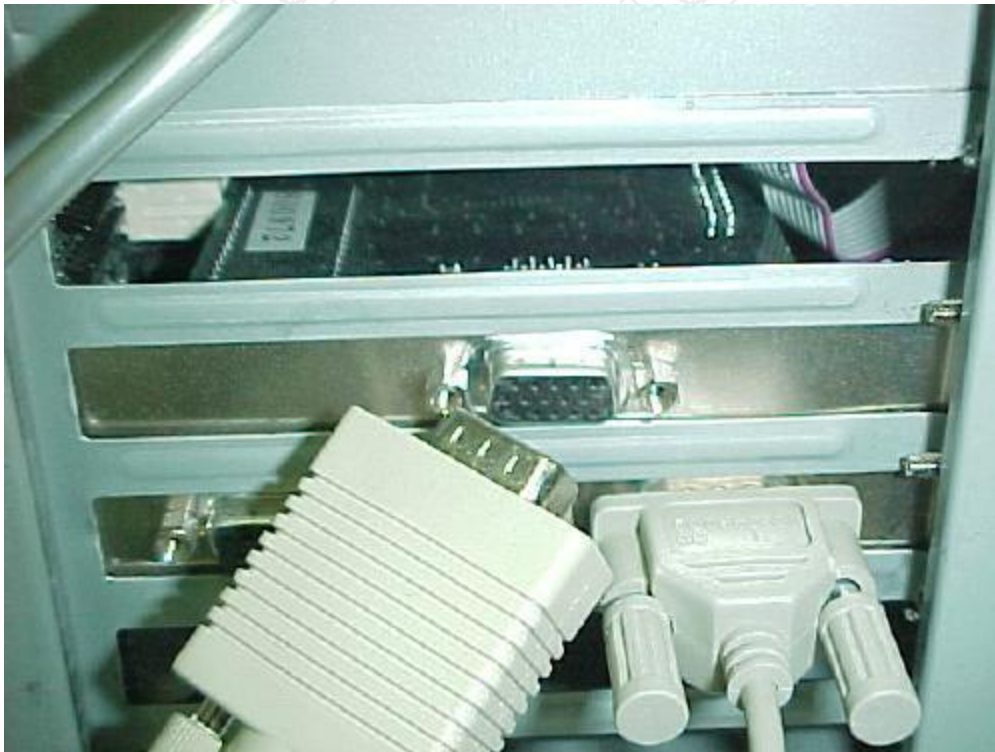
Figure 4 - The image above shows a close up of the monitor VGA connector at the rear of a computer after it has been removed from the video card VGA connector.
