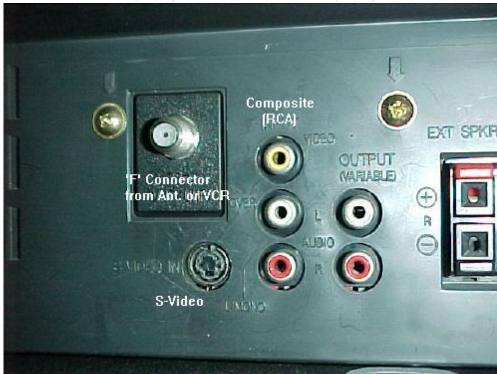
Figure 1 -The image above shows the rear panel of a television set. Note the labeling of the three connectors associated with the scan converter installation. You may have only one or two of these connectors on your TV.
