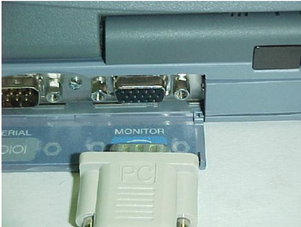
Figure 5 - The image above shows a close up of the VGA connector at the rear of a computer. The Pocket Scan Converter 2000 VGA connector is positioned for plugging into the computer VGA connector.
