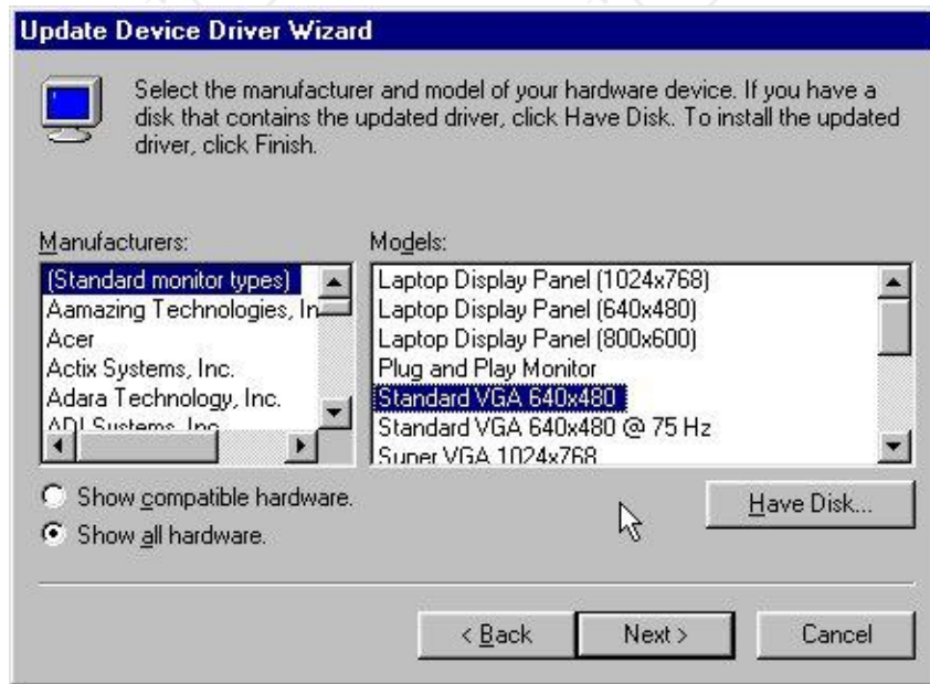
Figure 13 - Windows 98 Update Wizard (Win 95 Change Display Type) showing how to change display type.
