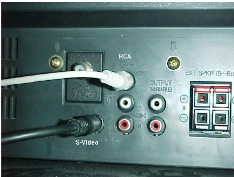
Figure 2 - Image showing the installation of the composite (RCA) video cable and the S-Video cable. Note: this is for illustration only - you will normally install one cable only.
