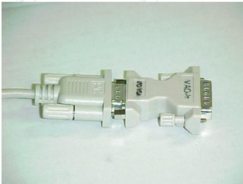
Figure 6 - Showing how to connect the Macintosh input adapter to the Pocket Scan Converter 2000 cable. The Mac In side of this connector connects to your Macintosh VGA (monitor) output connector
